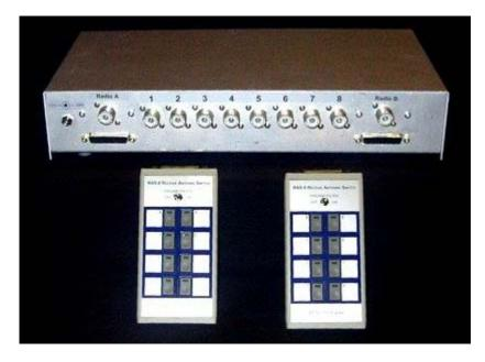
The RAS-8x2 provides flexible switching for your receiving antennas. Eight antennas can be routed to either of two radios, selected with remote keypads that fit easily into your shack. The standard preamp/filters for each radio provide 13-15 dB gain and filtering for 1.8-4.5 MHz (160M & 80M). When the preamps are OFF, the filters are also bypassed and the unit may be used on any frequency <0.5 MHz to 30 MHz.
